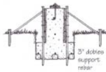
Fig. b1 • T Foundation with Forms
