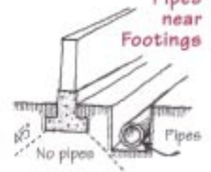
Fig. b3 Footings to Slope
